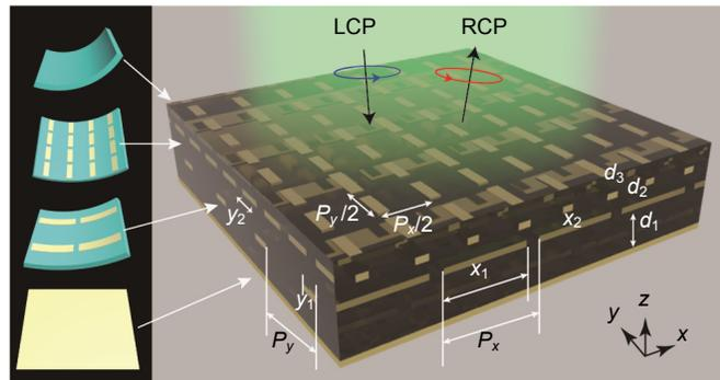
Fig.2 Schematic of the proposed anisotropic meta-mirrors for achromatic polarization manipulation, which is constructed by two meta-atoms array and a metallic reflection plane separated by dielectric spacers. The dielectric thicknesses from top to bottom are  $d_0$ ,  $d_1$  and  $d_2$ , respectively. The period of the metasurface is  $(P_x/2, P_y/2)$  and  $(P_x, P_y)$  for the upper one and bottom one, respectively.
