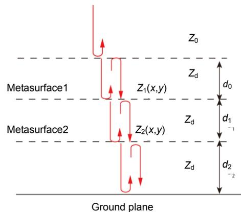
Fig.5 Schematic of the transmission line mode for achromatic polarization conversion.
