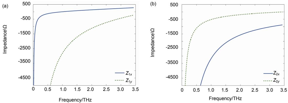
Fig.6 Retrieved impedance of (a) Metasurface 1 and (b) Metasurface 2 by equivalent circuit theory.
