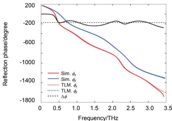
Fig.4 Simulated (solid line) and calculated (dash line) anisotropic dispersions of the metasurface and the phase difference  $\Delta\phi$ . TLM: transmission line model.
