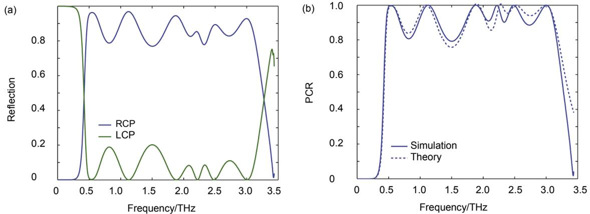
Fig.3 (a) Simulated reflectance of the co- and opposite- circular polarizations. (b) Simulated and theoretically calculated polarization conversion ratio.
