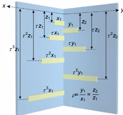
Fig.1 Schematic concept of wideband polarization-transforming electromagnetic mirror based on log-periodic antennas.
