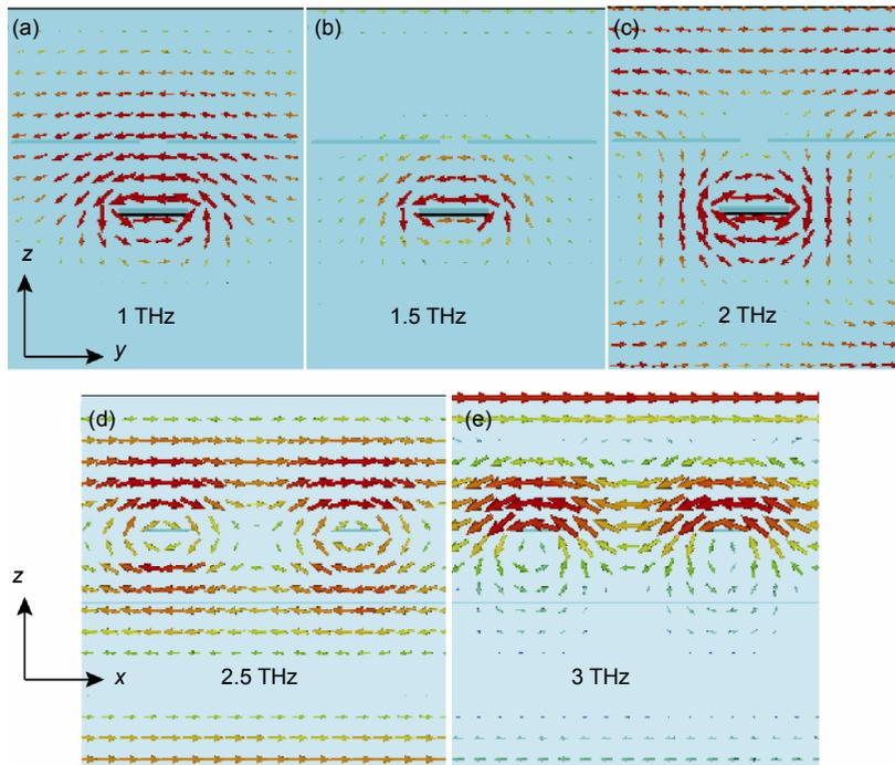
Fig.7 (a)–(e) Magnetic field distributions of the unit cell at frequencies of 1, 1.5, 2, 2.5 and 3 THz, respectively.
