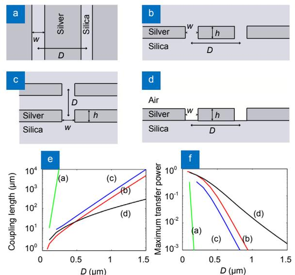
Fig. 1 | Four different waveguide schematics ((a), (b), (c), (d)) and the dependences of (e) coupling length  $L_c$  and (f) maximum transfer power  $P_{max}$  on separation distance  $D$ <sup>23</sup>.
