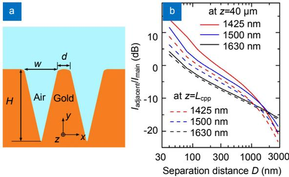
**Fig. 2 |** (a) The schematic of two adjacent parallel channel plasmon-polariton waveguides. (b) The crosstalk performance with specific parameters<sup>27</sup>.
