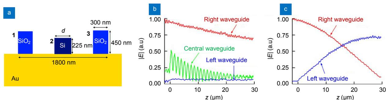
**Fig. 6 |** (a) The schematics of the surface plasmon waveguide system with the auxiliary waveguide. The distribution of the absolute values of the electric fields at waveguides (b) with and (c) without the auxiliary waveguide<sup>33</sup>.
