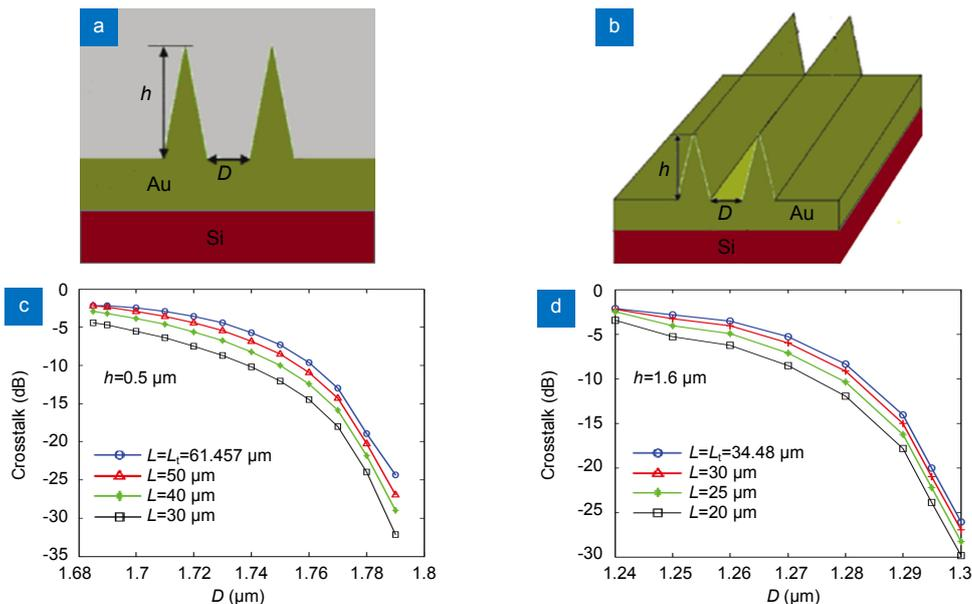
**Fig. 3 |** (a) The 2D and (b) 3D schematic diagrams of two WPP waveguides. Normalized crosstalk power of WPP waveguides under different parameters with wedge height (c)  $h=0.5 \mu\text{m}$  and (d)  $h=1.6 \mu\text{m}$ <sup>32</sup>.
