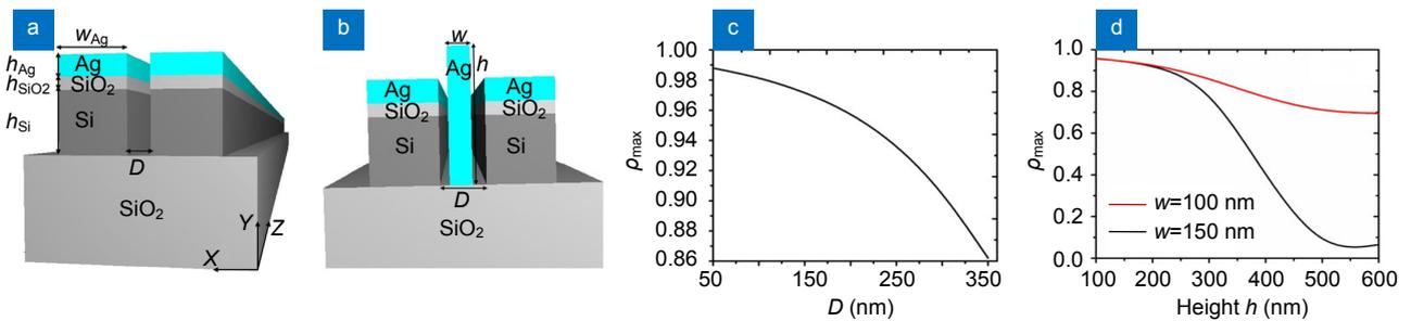
**Fig. 5 |** Schematic configuration of the two parallel hybrid silicon plasmonic waveguides (HSPW) (a) without and (b) with metallic strip. The maximum power transfer  $P_{max}$  versus specific parameters (separation distance  $D$ , height  $h$  and width  $w$  of the metallic strip) (c) without and (d) with metallic strip<sup>30</sup>.
