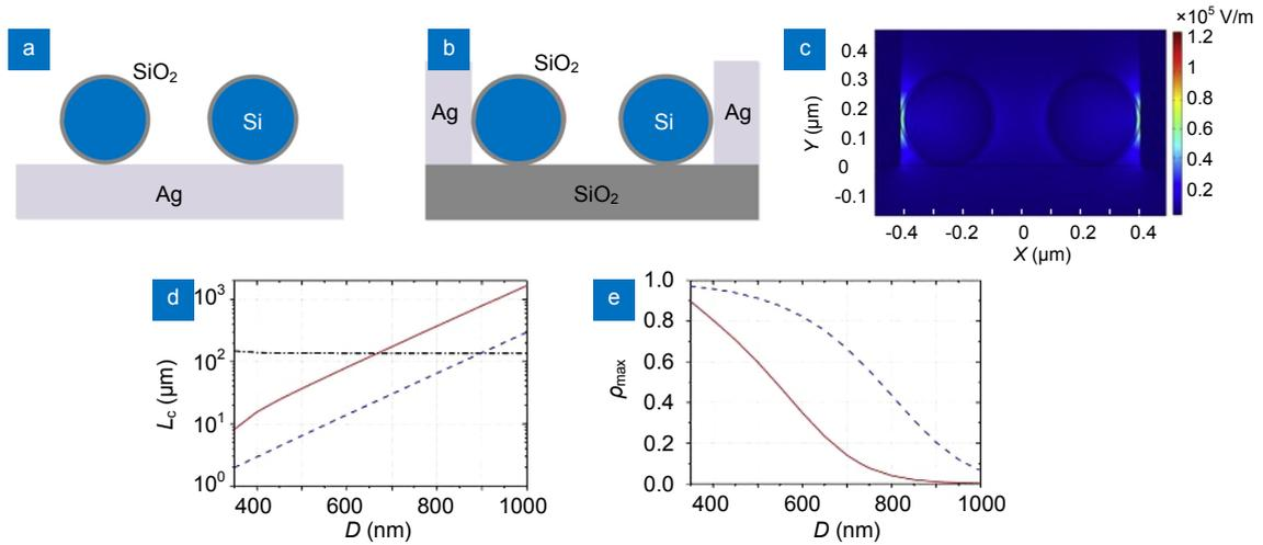
**Fig. 4 |** Schematic diagrams of (a) hybrid waveguide and (b) its rotation, (c) distribution of  $E$ , field for rotation hybrid waveguide, (d) coupling length  $L_c$  and (e) maximum power transfer  $P_{max}$  as functions of the separation  $D$ , the red solid line and blue dotted line represent the results of the two structures of (a) and (b), respectively<sup>25</sup>.
