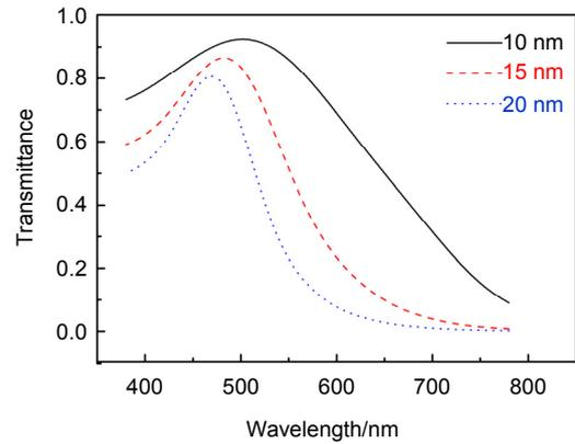
Fig. 2 Optical transmission spectra simulated using FDTD for normal incidence with 3.5 pairs of layers consisting of 10 nm, 15 nm and 20 nm Ag films respectively, and a fixed ITO films thickness at 60 nm transmittance
