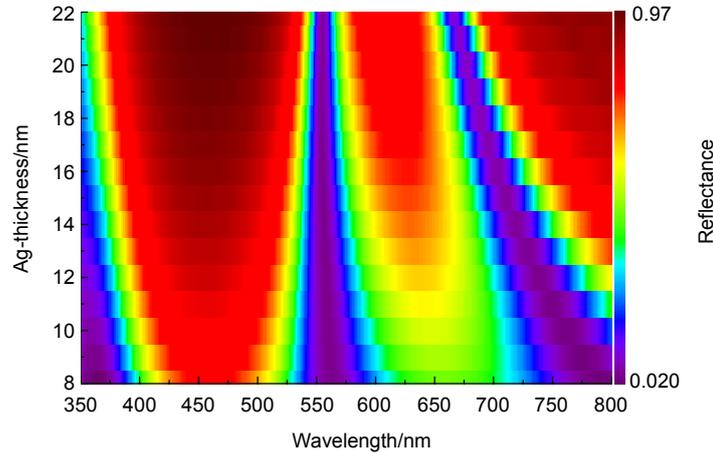
Fig. 8 Optical reflection spectra simulated using FDTD for normal incidence with 3.5 pairs of Ag/ITO with a Ag layer ranging from 8 nm to 22 nm and ITO films of 120 nm thickness
