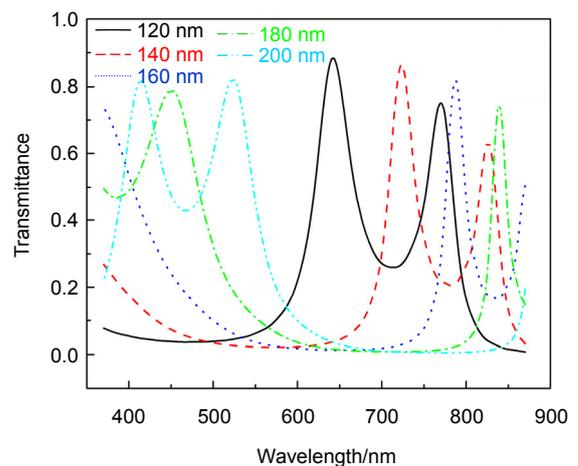
Fig. 5 Optical transmission spectra simulated using FDTD for normal incidence with 3.5 pairs of Ag/ITO layers consisting of 120 nm, 140 nm, 160 nm, 180 nm, and 200 nm ITO films, respectively, and a fixed Ag films thickness of 20 nm
