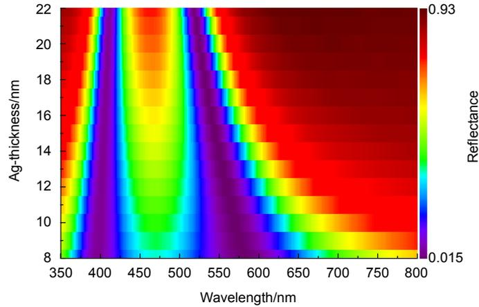
Fig. 7 Optical reflection spectra simulated using FDTD for normal incidence with 3.5 pairs of Ag/ITO with a Ag layer ranging from 8 nm to 22 nm thickness and fixed ITO thickness of 80 nm
