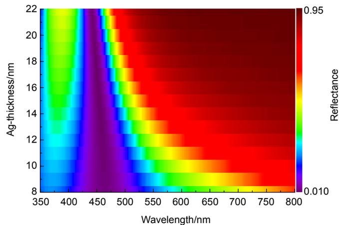
Optical reflection spectra simulated using FDTD for normal incidence with 3.5 pairs of Ag/ITO, consisting of Ag with thicknesses from 8 nm to 22 nm, and a fixed ITO thickness of 60 nm
