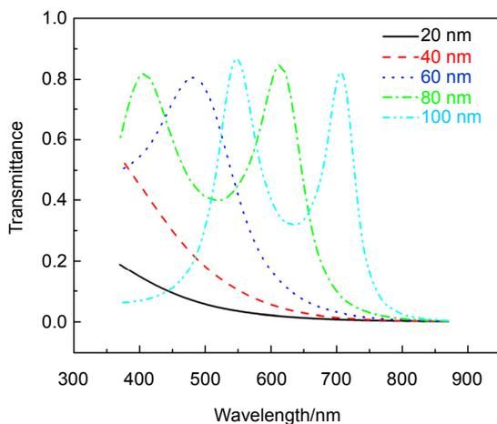
Fig. 4 Optical transmission spectra simulated using FDTD for normal incidence with 3.5 pairs of Ag/ITO, which consist of 20 nm, 40 nm, 60 nm, 80 nm and 100 nm ITO films, respectively, and fixed Ag films of 20 nm thickness
