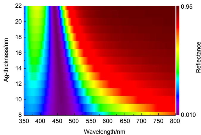
Fig. 6 Optical reflection spectra simulated using FDTD for normal incidence with 3.5 pairs of Ag/ITO, consisting of Ag with thicknesses from 8 nm to 22 nm, and a fixed ITO thickness of 60 nm
