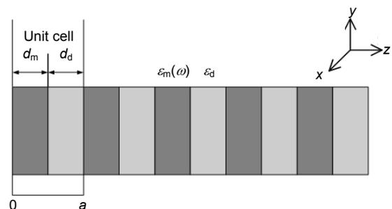
Fig. 1 Structure of the Ag-PBG with 3.5 pairs
