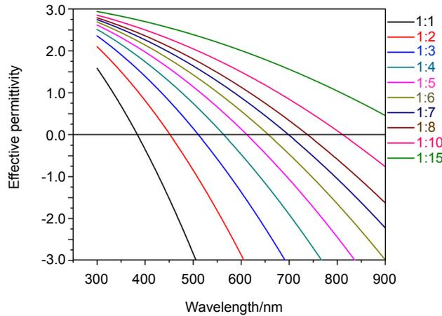
Fig. 3 Calculated effective permittivity for a ratio of Ag to ITO thickness of 1:1, 1:2, 1:3, 1:4, 1:5, 1:6, 1:7, 1:8, 1:10 and 1:15, according to equation (3)
