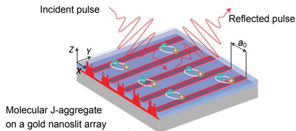
Schematic of coherent ultrafast spectroscopy on a hybrid nanostructure consisting of a 50-nm-thick film of J-aggregate molecules in a polymer matrix coated onto a gold nanogroove array with period  $a_0$ . Strongly localized SPP fields (in red) exist in and near the grooves. Incident and reflected laser pulses and J-aggregate excitons are shown schematically.
