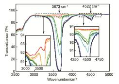
Transmittance spectra of 9 fused silica samples with 2.0 mm thickness at 2500 cm<sup>-1</sup>~5000 cm<sup>-1</sup> wavenumber measured 30 times. The results show Si—OH absorption bands with the absorption intensity becoming smaller: Infrasil 302, HOQ 310, Suprasil 711, Suprasil 501, Herasil 3, Suprasil 401, Herasil 102, Corning 7980, Spectrosil 2000.
