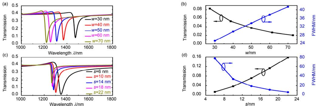
Transmission spectra of (a) different resonator width (c) different coupling distance. Transmission dip wavelength and FWHM as a function of (b) resonator width  $w$ , and (d) coupling distance  $s$ . Here,  $L_1=L_2=420$  nm,  $s=10$  nm,  $h_1=170$  nm,  $h_2=120$  nm, and  $w=50$  nm.
