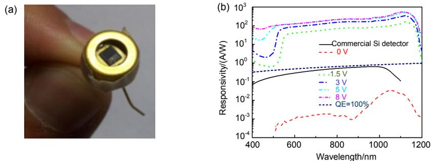
Picture of photodetector (a) and (b) responsivities as a function of applied bias voltage for a sulfur-hyperdoped silicon photodiode.
