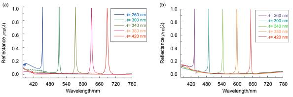
Fig. 2 Reflection spectra of the GMRF with  $\Lambda$  of 260 nm, 300 nm, 340 nm, 380 nm and 420 nm. (a) TE polarization. (b) TM polarization.
