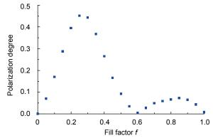
Fig. 5 Polarization degree of the reflected light of GMRF with different fill factors.
