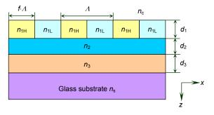
Fig. 1 Structure of a triple-layer GMRF.
