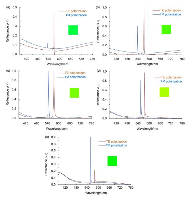
Fig. 4 Reflection spectra and colors of the GMRF with f of (a) 0.1, (b) 0.25, (c) 0.5, (d) 0.75 and (e) 0.9.
