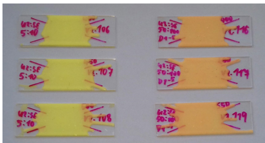
Fig. 2 | Photograph of a microscope slide containing emitting samples with PDMS and YAG:Ce 3+ (main emission peak at 555 nm) on the left side and the samples on the right side contain PDMS, YAG:Ce 3+ and CaS:Eu 2+ (main emission peak at 650 nm), using as excitation source blue light. Figure reproduced from ref. 37 , under a Creative Commons Attribution International License.
