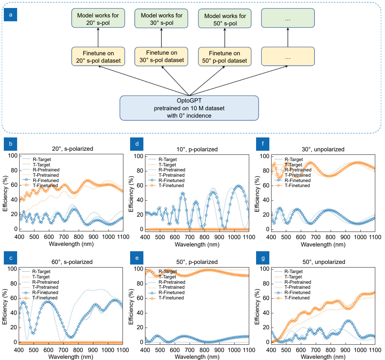
Fig. 7 | Design performance on different angles and polarization. (a) The diagram of finetune. (b–g) gives inverse design examples for spectrum with 20° s-polarization, 60° s-polarization, 10° p-polarization, 50° p-polarization, 30° unpolarized and 50° unpolarized, respectively. The solid line, dashed line and squared line correspond to the target spectrum, spectrum designed by the pretrained model and spectrum designed by the finetuned model, respectively.
