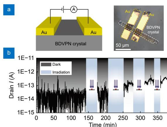
**Fig. 4 |** Enhancement of charge transport under irradiation. (a) Schematic and optical microscope images of the electrical device, two Au film electrodes were transferred to the crystal. (b) The evolution of dark current (at a 60 V applied voltage) of the BDVPN crystal over time before and after the irradiation treatment (405 nm CW laser,  $60 \text{ mW}\cdot\text{cm}^{-2}$ ).
