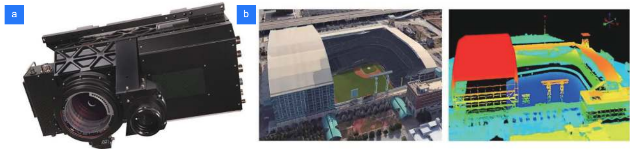
图 16 徕卡 SPL100 与获取的地物信息 [57] 。(a) 徕卡 SPL100 系统; (b) SPL100 重建结果 Fig. 16 The Leica SPL100 system and terrain features acquired by the SPL100 [57] . (a) The Leica SPL100 system; (b) Results reconstructed by the SPL100
