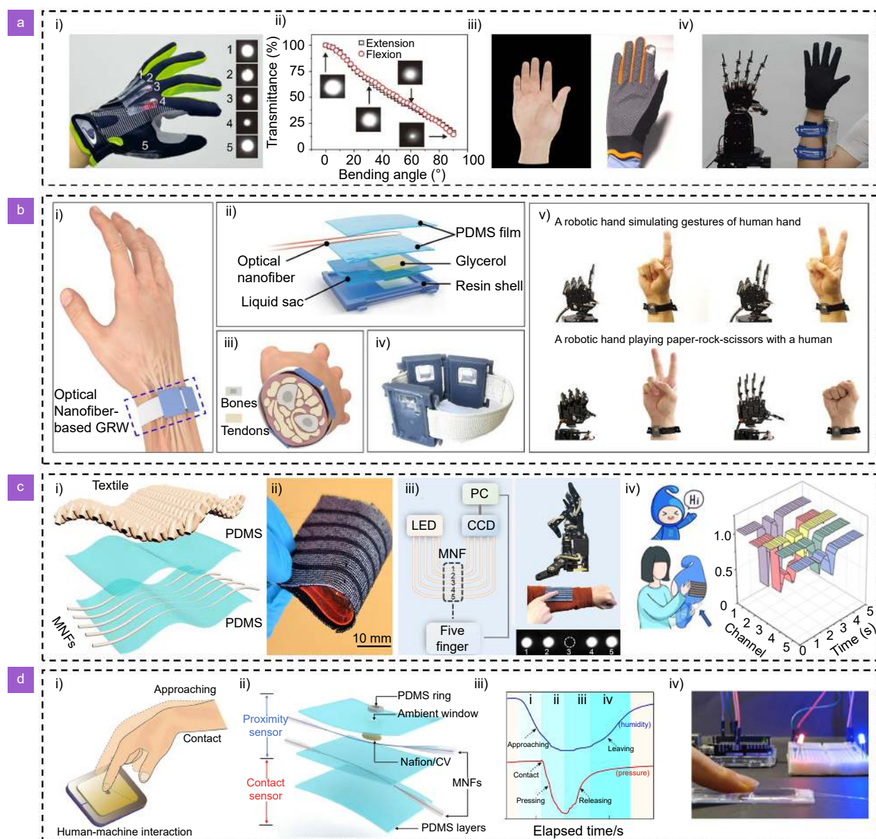
Fig. 5 | MNF tactile sensors for human machine interaction. (a) MNF bending sensor enabled data gloves. i) Image of an MNF glove with five bending sensors; ii) Bending-angle-dependent output of a typical MNF bending sensor; iii) Image of a virtual hand controlled by an MNF data glove; iv) Image of a robotic hand controlled by an MNF data glove. Figures reproduced with permission from ref. 28 , under a Creative Commons Attribution 4.0 International License. (b) MNF pressure sensor enabled wristband. i) Schematic of the MNF enabled wristband; ii) Schematic of the MNF pressure sensor; iii) Cross-section of a wrist with a three-sensor wristband, indicating the position of the sensors and tendons; iv) Photograph of a three-sensor wristband; v) Application of the wristband for controlling a robotic hand based on hand gesture recognition. Figures reproduced with permission from ref. 120 , under a Creative Commons Attribution License. (c) MNF pressure sensor enabled smart textiles. i) Schematic of optical MNF enabled smart textiles. ii) Optical image of the as-fabricated smart textiles. iii) Logic control of a robotic hand via the smart textile. iv) Machine learning enabled emotional human machine interface. Figures reproduced with permission from ref. 122 , © 2022 Donghua University, Shanghai, China. (d) MNF humidity and pressure sensor enabled contact and proximity sensing. i) Schematic diagram of contact and proximity interaction; ii) Schematic of the contact and proximity sensor; iii) Responses of the sensor under finger approaching and contacting; iv) Photograph of the contact and proximity switch system for controlling the on/off of the LEDs. Figures reproduced with permission from ref. 125 , © 2022 American Chemical Society.
